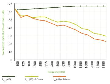
Normalized impact sound pressure level of the Lab reference floor:
